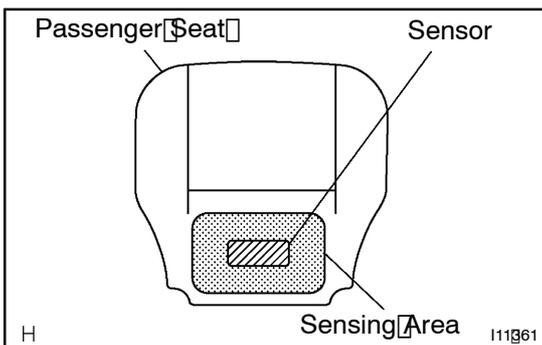
**28. Passenger seat only: INSPECT SEAT BELT WARNING OCCUPANT DETECTION SENSOR CONTINUITY**
