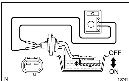
(c) Check that there is continuity between terminals with the switch ON (float down).
